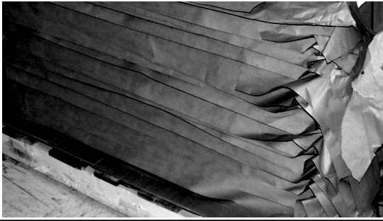
Exhibit 3: Panel assemblies are separated only with Kraft paper. Once the assemblies are deunitized and subsequently delivered to GSI Lumonics inventory, they are at risk of surface damage through normal material
