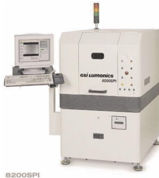
Figure 1 is an illustration of a typical in-line system using a laser scanner for component placement inspection. During inspection, the board is held still. The system projects a very low powered laser onto the PCB and measures the position of the reflected beam
