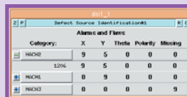
FIGURE C: The detail from a selected bar in Figure B relates measurement data back to the performance of the placement equipment.
