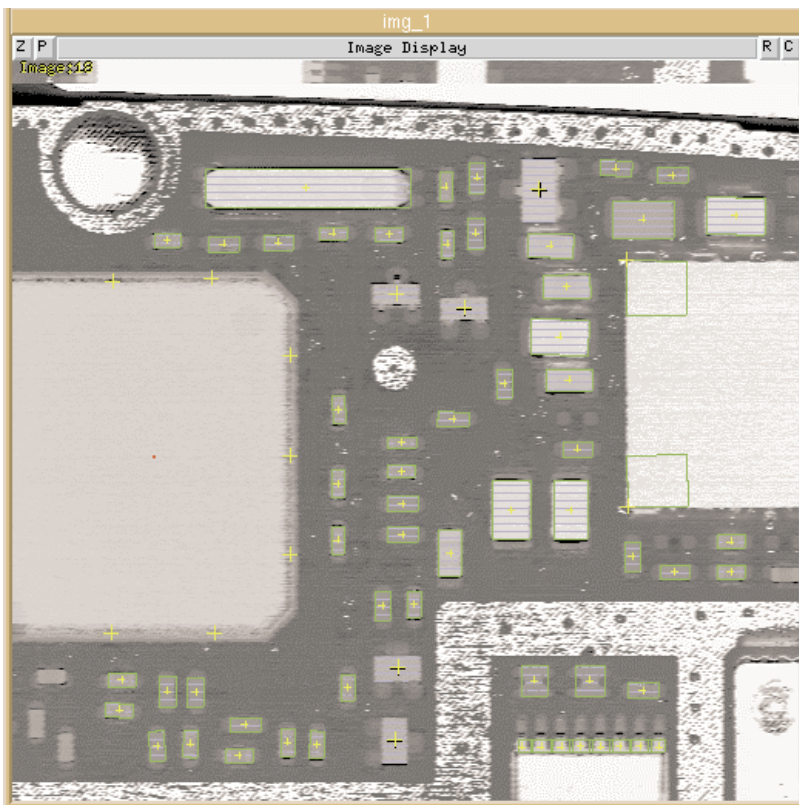
as chip resistors is when they appear the same greyscale as the board.
